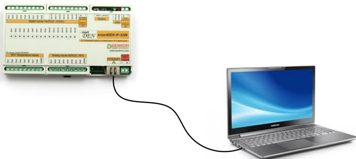
Figure 5.10. Connecting smartDEN IP-32IN-XX to a computer directly. This is the recommend initial connection
