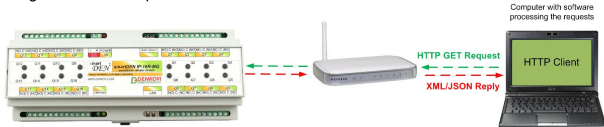
Figure 9.1. smartDEN IP-16R-XX working as a HTTP server
