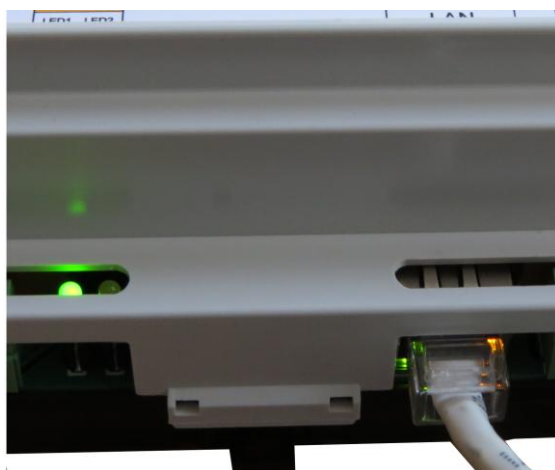
Figure 6.3. Connecting a LAN cable
