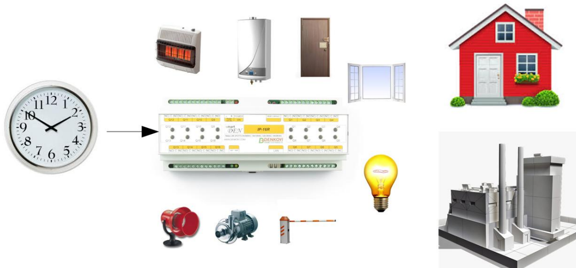
Figure 3.1. smartDEN IP-16R-XX supports up to 30 schedule events for controlling appliances without connection with computer.
