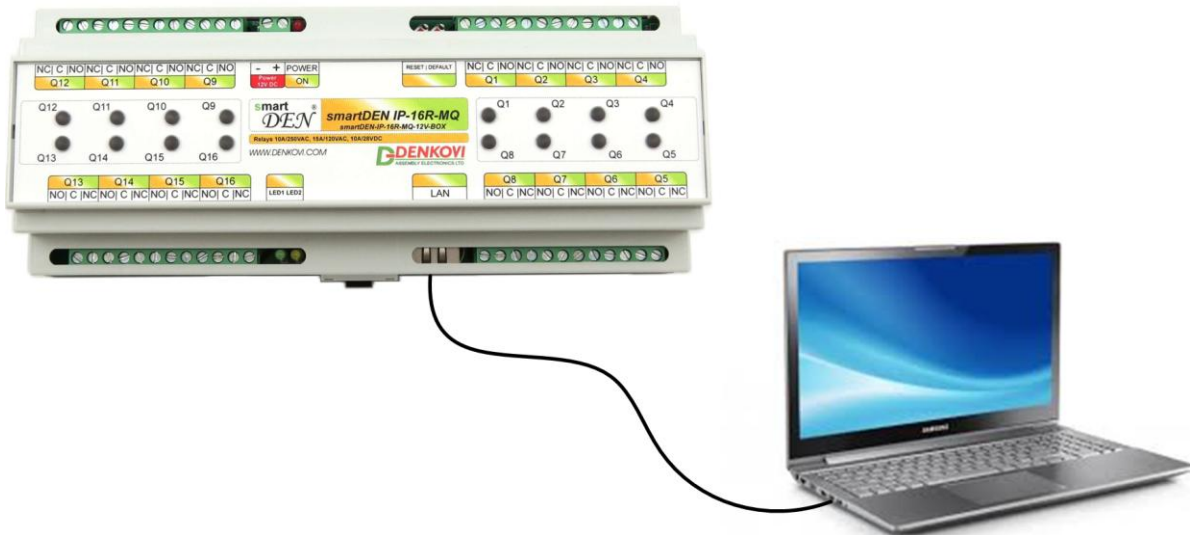
Figure 6.5. Connecting smartDEN IP-16R-XX to a computer directly. This is the recommend initial connection.
