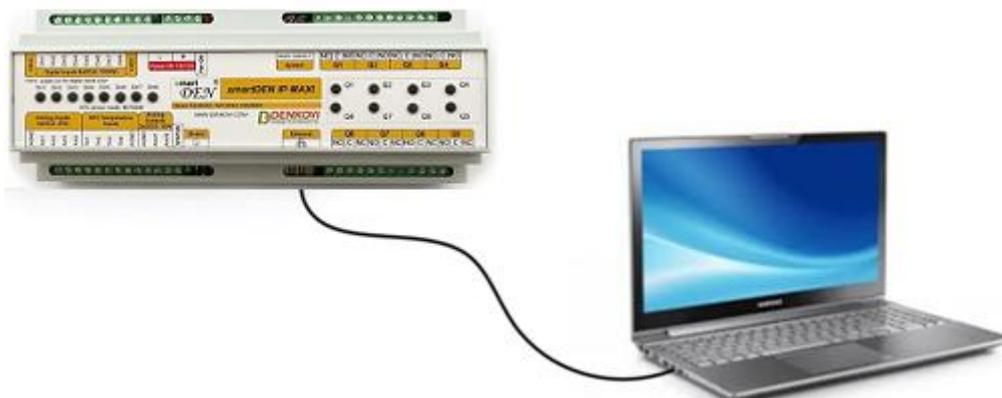
Figure 5.10. Direct connection of smartDEN IP-Maxi to a computer
