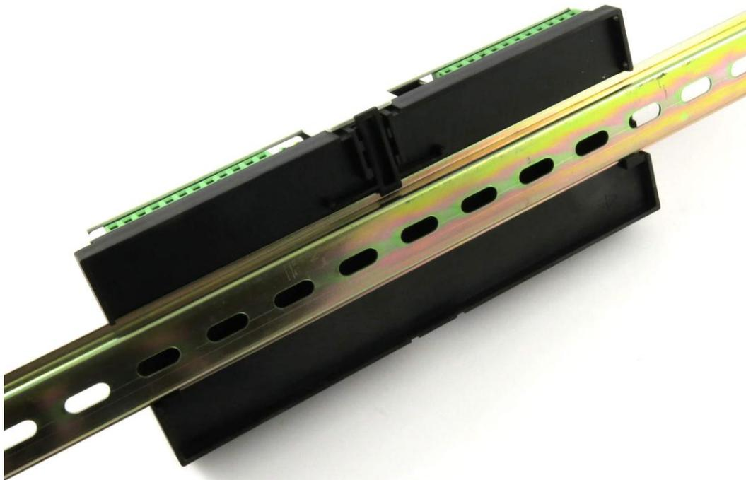
**Figure 5.1.** Mounting the device to a DIN rail
