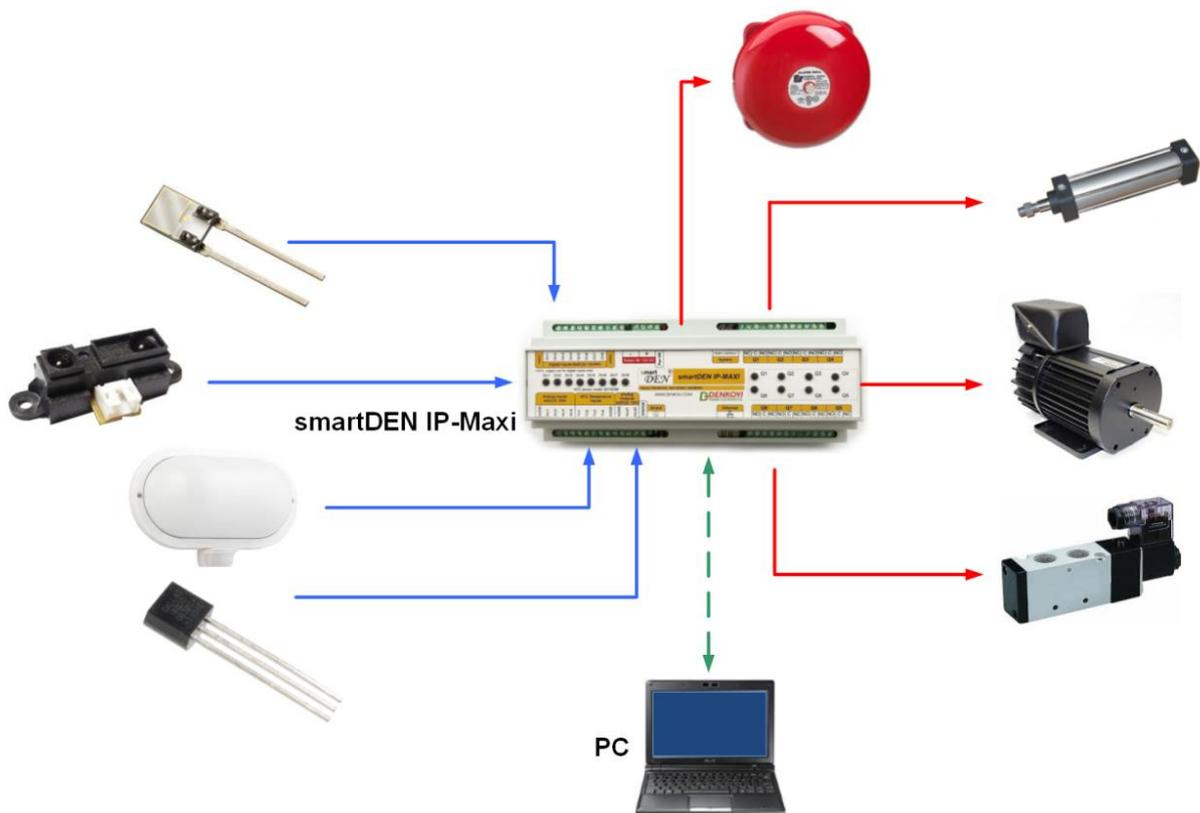
Figure 2.3. Standalone control of electrical devices
