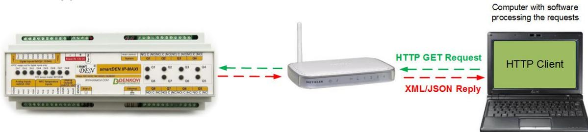
**Figure 8.1. smartDEN IP-Maxi working as a HTTP server**
