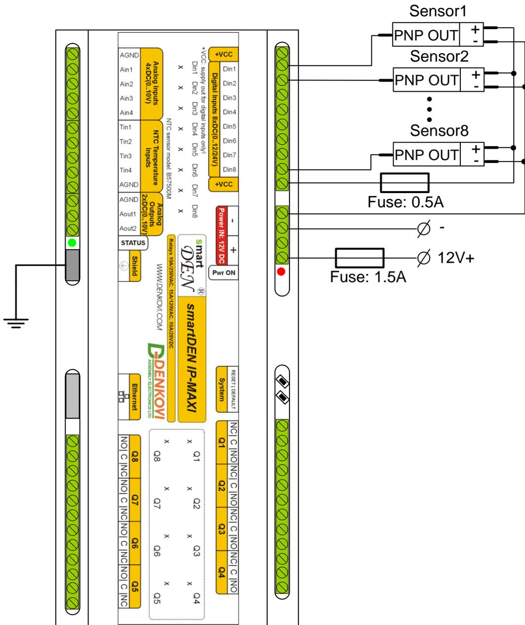
**Figure 5.4.** Connecting PNP output digital sensors requiring power supply voltage 12V DC to the Digital Inputs
