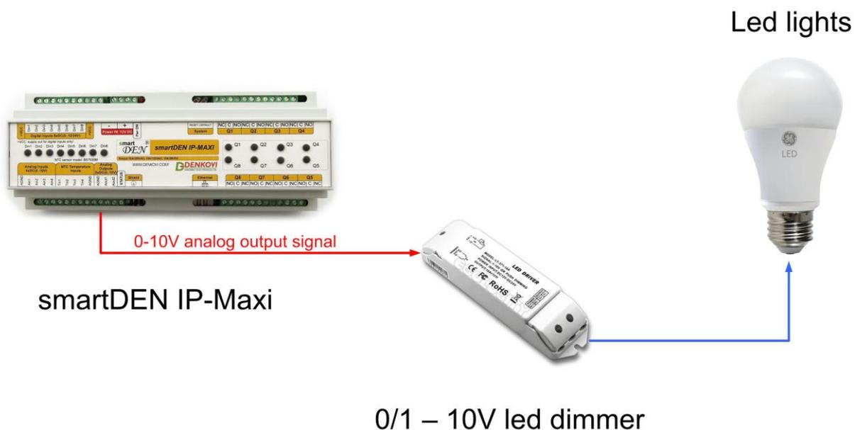
Figure 5.9. Controlling led lights with analog outputs
