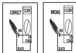
Figure 16. Correct polarity
