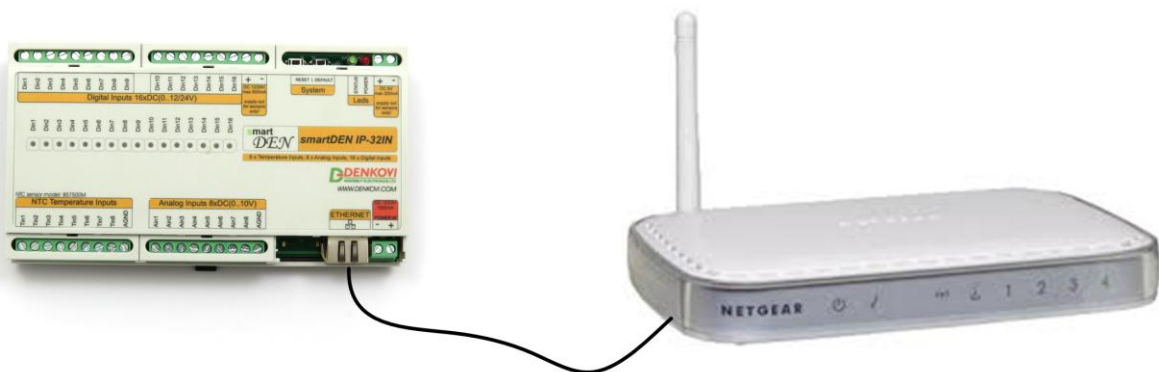
Figure 15. Connecting SmartDEN IP-32IN to a wireless router
