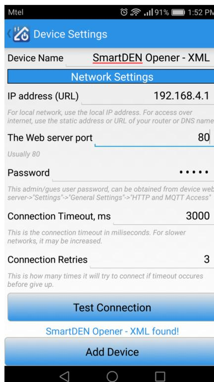
Figure 6.28. smartDEN Opener - XML Settings
