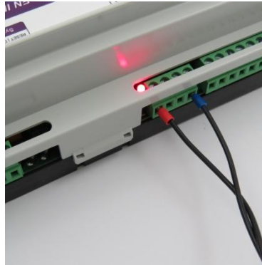
Figure 5.2. smartDEN IP-PLC power supply
