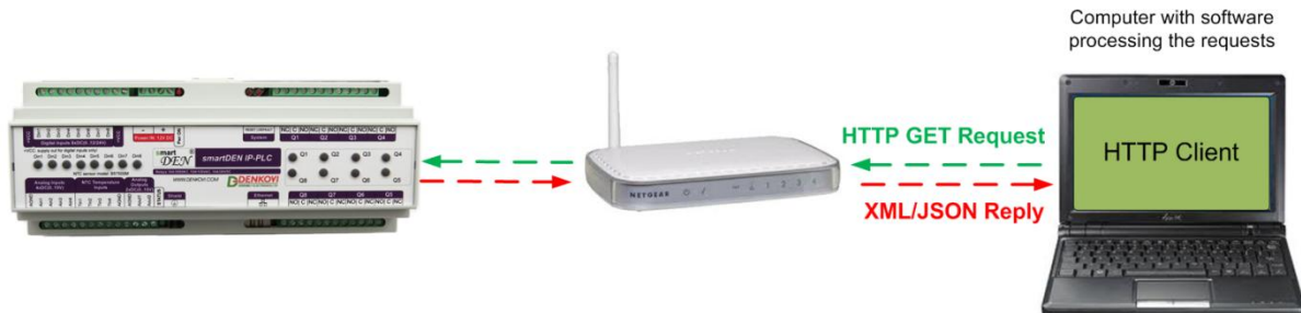
Figure 10.1. smartDEN IP-PLC working as a HTTP server
