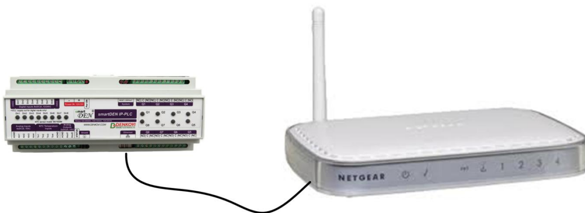
Figure 5.11. Connecting smartDEN IP-PLC to a wireless router
