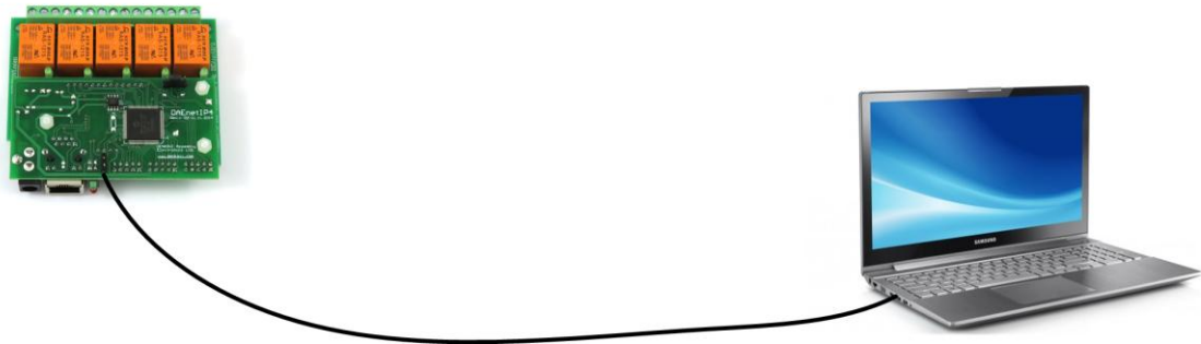
Figure 13. Connecting DAEnetIP4 Five Relay Module to a computer directly (recommended initial connection)
