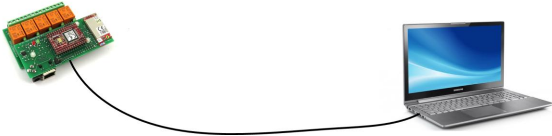
Figure 10. Connecting DAEnetIP3 Five Relay Module to a computer directly (recommended initial connection)
