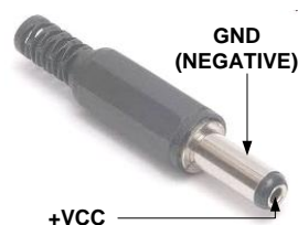
Figure 7. How the power supply cable must look like
