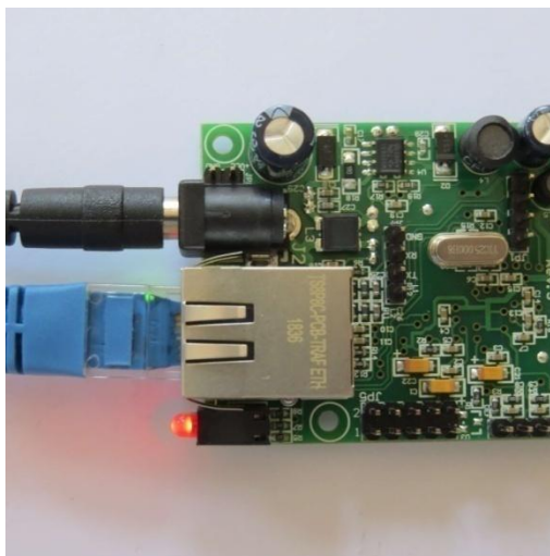
Figure 12.9. Plug the power supply jack into DAEnetIP2 v2
