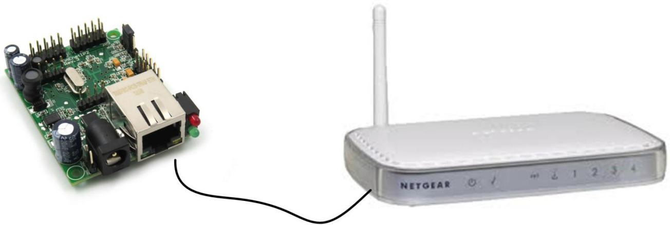
Figure 11.2. DAEnetIP2 v2 connected to router
