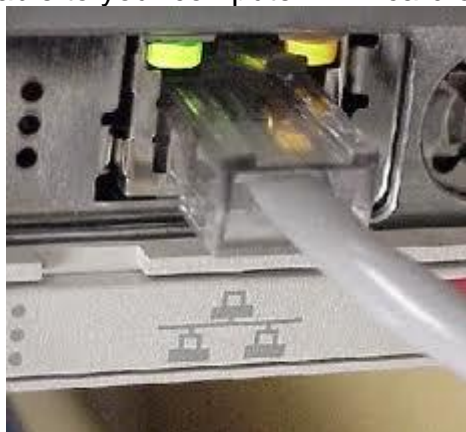
Figure 12.2. Connecting UTP cable to Computer
