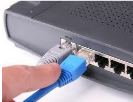
Figure 12.3. Connecting UTP cable to router
