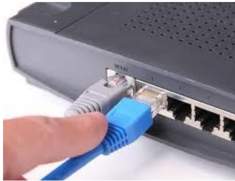
Figure 20. Connecting UTP cable to router
